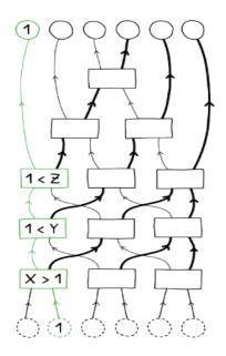
Repeat this until you've tested all 6 nodes. If the smallest number ends up in the leftmost node regardless of where it starts, that's part-way to being sure that the structure always works.
